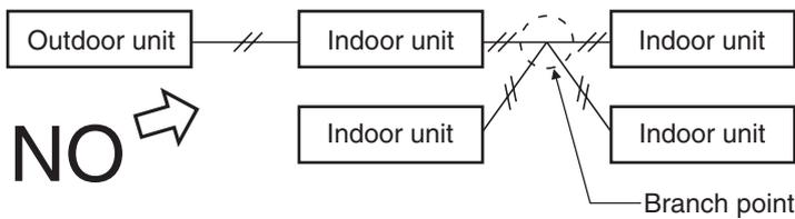
**(4) If branching the inter-unit control wiring, the number of branch points should be 16 or fewer.**
