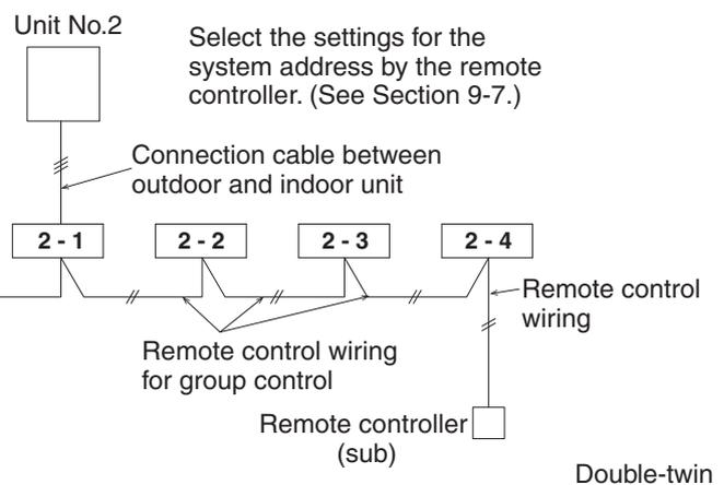
\* If two (2) remote controllers are used, one (1) remote controller is set to “main” and the other is set to “sub”. (See Section 9-11.)
