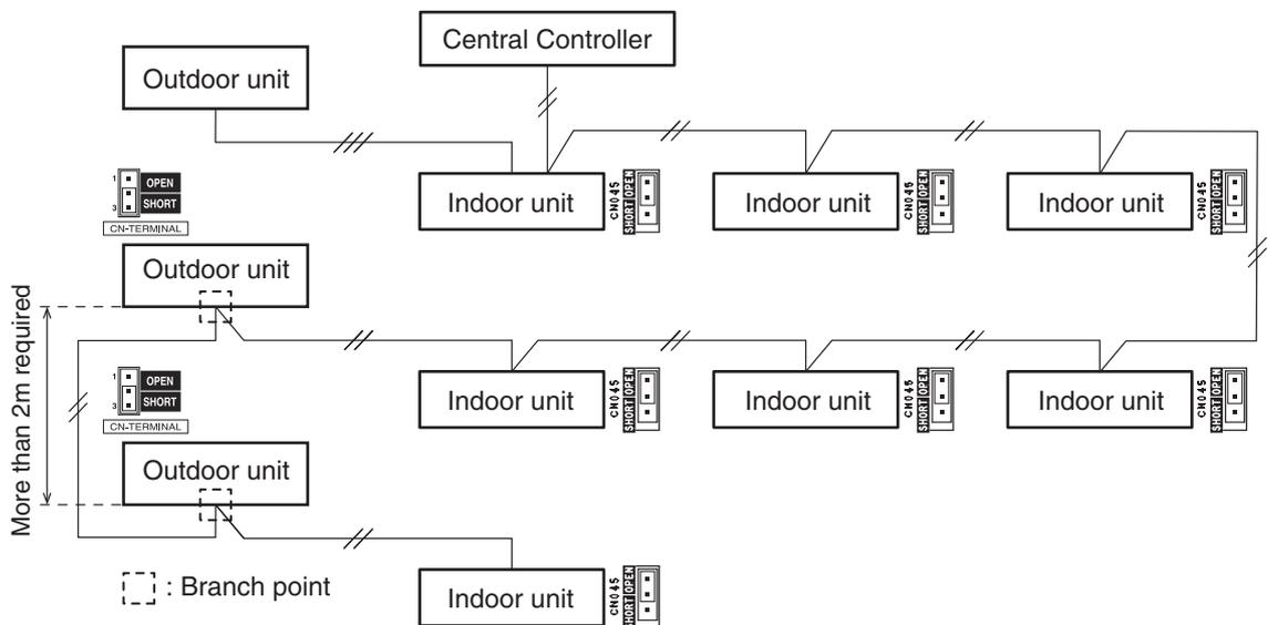
(5) Use shielded wires for inter-unit control wiring (C) and ground the shield on both sides, otherwise misoperation from noise may occur. Connect wiring as shown in Section 4-3.
