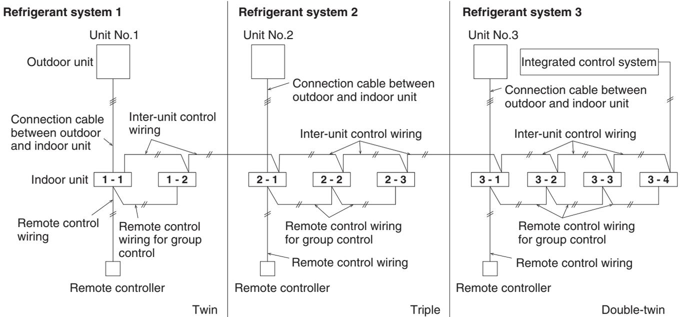
\* It is possible to connect maximum 8 indoor units with one remote controller.
