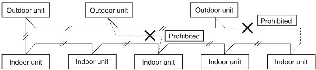
**(3) Do not install inter-unit control wiring such as star branch wiring. Star branch wiring causes mis-address setting.**
