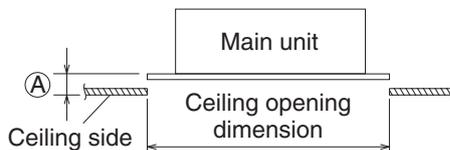
Ⓐ :Be sure to necessarily make a space within the range of 13 mm ~ 18 mm.
