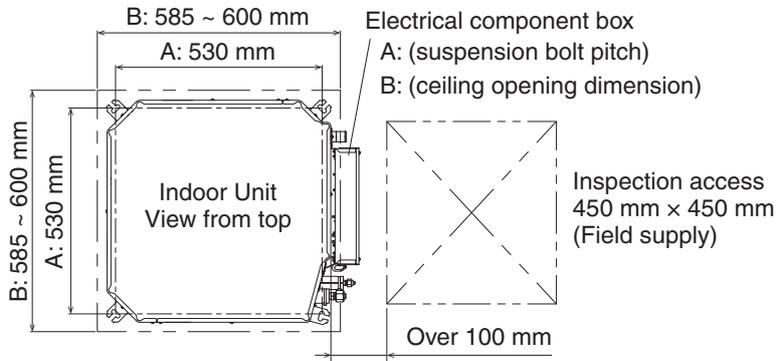
(3) Determine the pitch of the suspension bolts using the supplied full-scale installation diagram (printed on container box). The diagram show the relationship between the positions of the suspension fitting, unit, and panel. Use the nut (field supply) and washer (supplied) for upper and lower position of the suspension lug.
