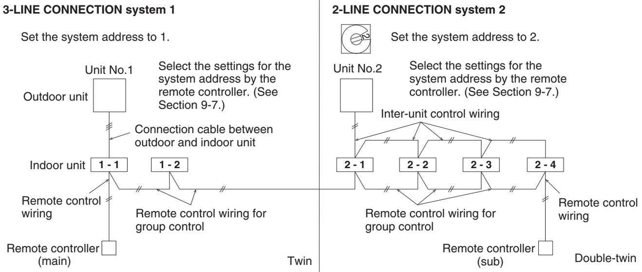
\* If two (2) remote controllers are used, one (1) remote controller is set to “main” and the other is set to “sub”. (See Section 9-11.)
