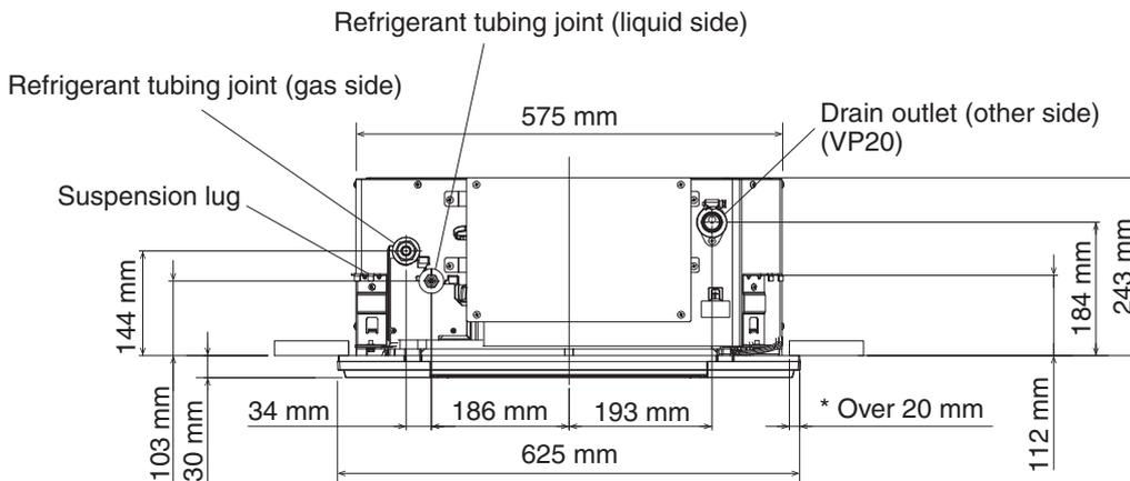
\* The overlapping portion between the ceiling and panel for cassette should be kept over 20 mm.
