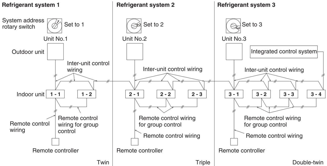
\* It is possible to connect maximum 8 indoor units with one remote controller.
