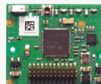
Wireless ZigBee® Pro module / Green Com card.
