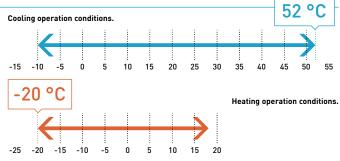
Cooling: Outside air temperature  $^{\circ}$ C (DB). Heating: Outside air temperature  $^{\circ}$ C (WB).
