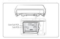
**4** Find the PCB wire, and connect the wire to the Sub PCB as seen in the picture.
