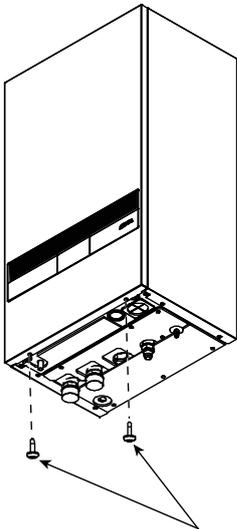
1. Remove the 2 mounting screws which located at bottom of the front plate.
