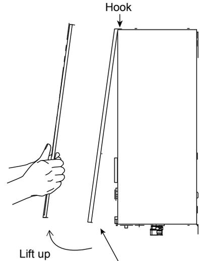
3. Hold the left edge and right edge of front plate to lift up front plate from hooks.
