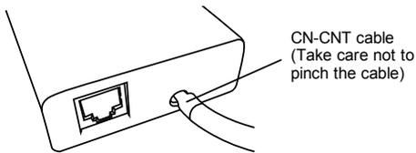
4. Fix the Network Adaptor 8 to Network Adaptor Holder. Guide the cable as shown in the diagram so that external forces cannot act on the connector in the adaptor.
