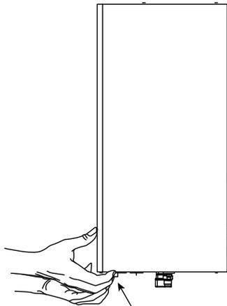
2. Gently pull the lower section of the front plate towards you to remove the front plate from left and right hooks.
