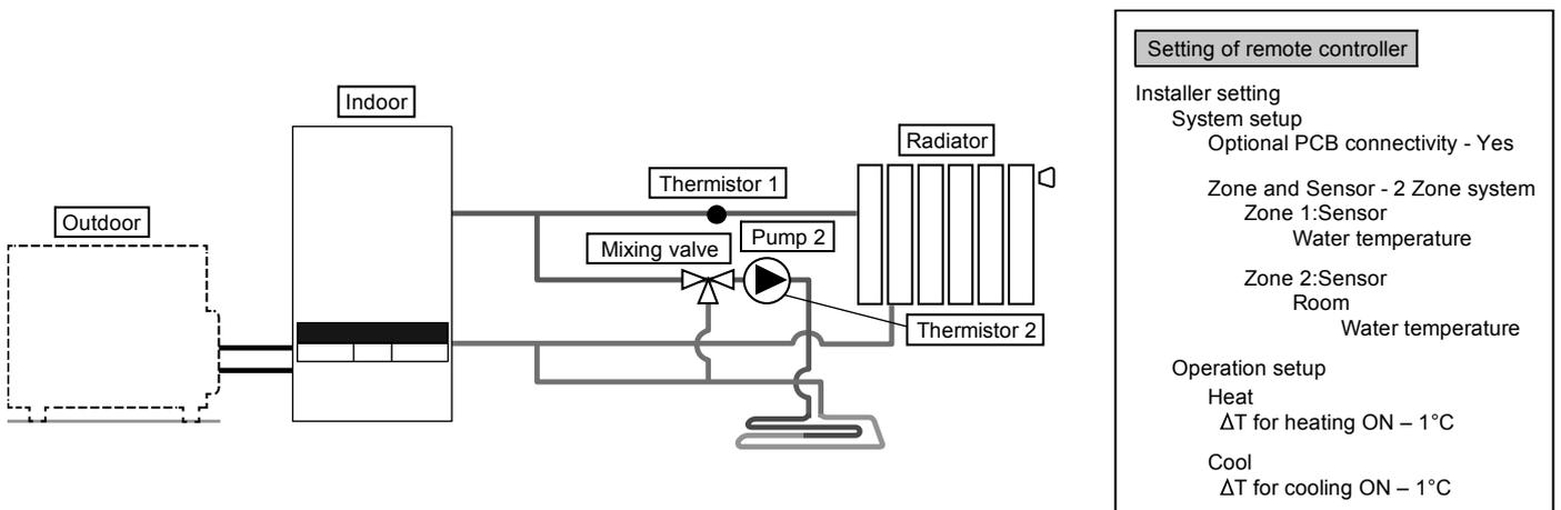
This is an example of simple 2 zone control without using buffer tank.
