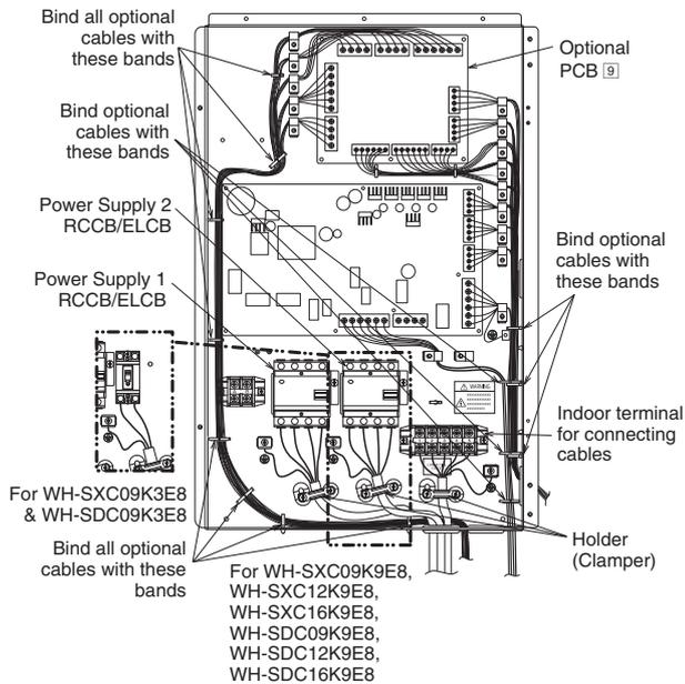
How to guide the optional cables and power supply cord (view without internal wiring)
