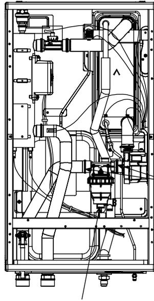
2. Disconnect 2 pipes connection.
