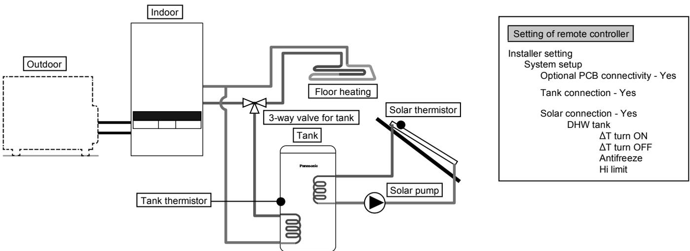
This is an application that connects the DHW tank to the Indoor Unit through 3-way valve before connect the solar water heater to heat up the tank. DHW tank's temperature is detected by tank thermistor (specified by Panasonic).
