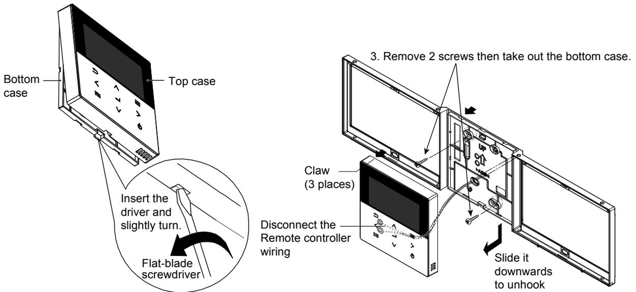
1. Remove the top case from the bottom case.
