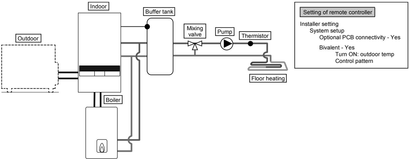
This is an application that connects the boiler to the Indoor Unit, to compensate for insufficient capacity by operate boiler when outdoor temperature drops & heat pump capacity is insufficient.
