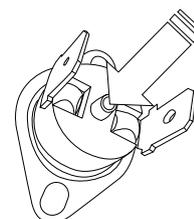
Use test pen to push this button for reset Overload protector ⑪.
