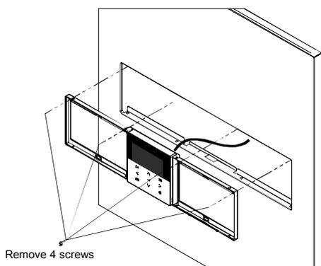
3. Remove the top case from the bottom case.
