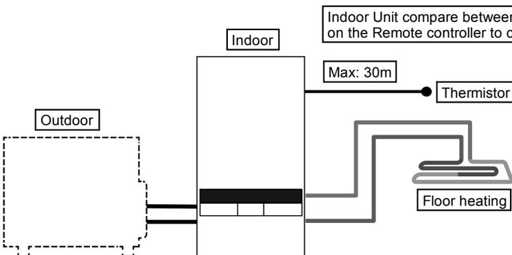
Indoor Unit compare between room temperature and setting temperature on the Remote controller to control HP and circulation pump.
