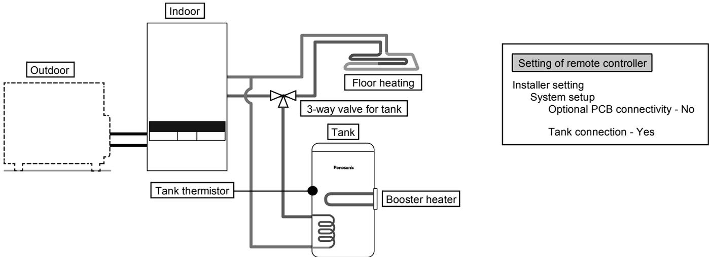
This is an application that connects the DHW tank to the Indoor Unit through 3-way valve. DHW tank's temperature is detected by tank thermistor (specified by Panasonic).
