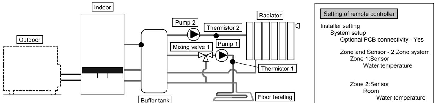
Connect floor heating or radiator to 2 circuits through buffer tank as shown in figure.
