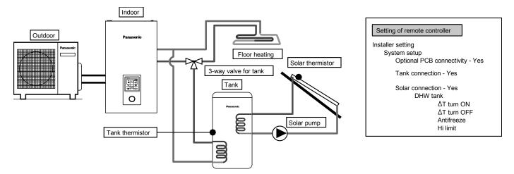
This is an application that connects the DHW tank to the indoor unit through 3-way valve before connect the solar water heater to heat up the tank. DHW tank's temperature is detected by tank thermistor (specified by Panasonic). Solar panel's temperature is detected by solar thermistor (specified by Panasonic).
