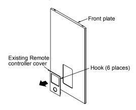
2. Press from front to fix the Remote controller cover on the front plate.
