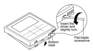
Remove the wiring between Remote controller and Indoor Unit terminal. Remove the bottom case from the Control board cover by loosening the screws. (2 pieces)
