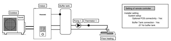
This is an application that connects the buffer tank to the indoor unit.
