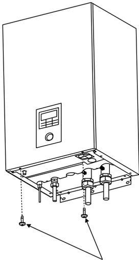
1. Remove the 2 mounting screws which located at bottom of the front plate.
