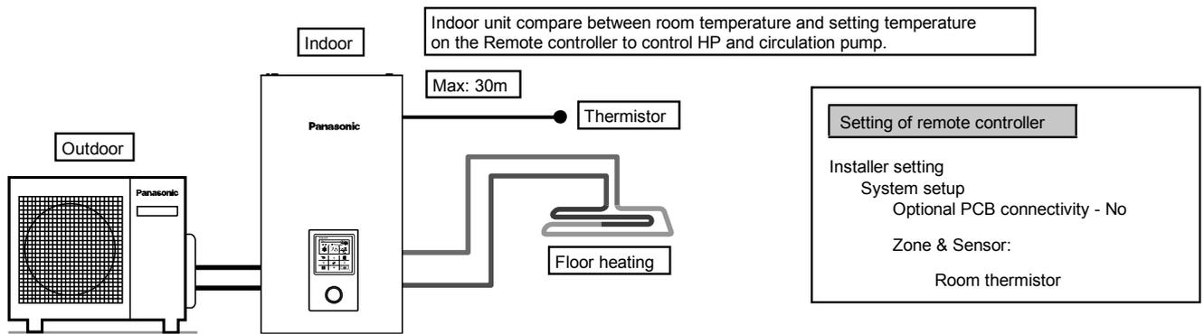
Connect floor heating or radiator directly to indoor unit.
