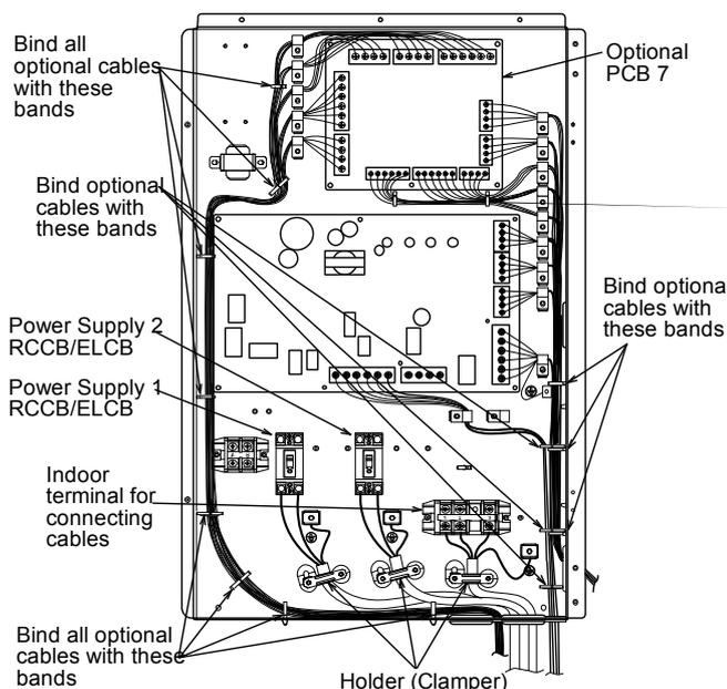
How to guide the optional cables and power supply cord
