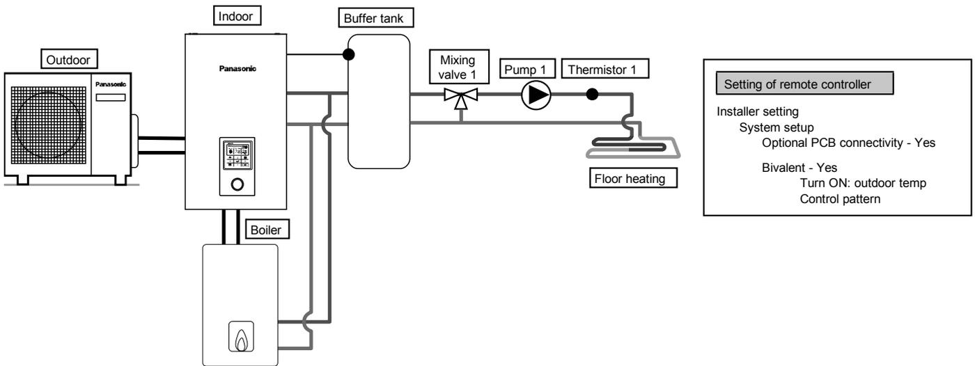
This is an application that connects the boiler to the indoor unit, to compensate for insufficient capacity by operate boiler when outdoor temperature drops & heat pump capacity is insufficient.
