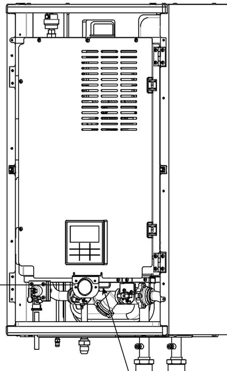
2. Use spanner to release nut of pressure gauge
