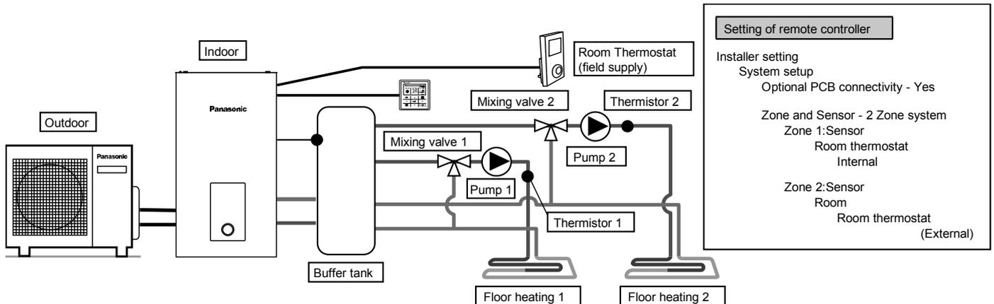
Connect floor heating to 2 circuits through buffer tank as shown in the figure.
