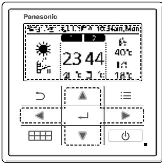
Press (☰ + ▼ + ◀) SW's continuously for 5secs
