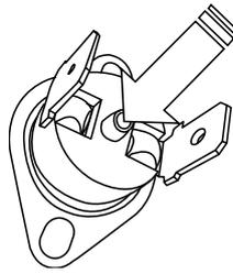
Use test pen to push this button for reset Overload protector.
