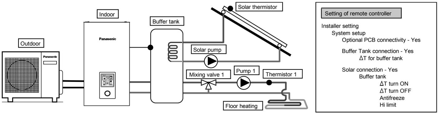
This is an application that connects the buffer tank to the indoor unit before connecting to the solar water heater to heat up the tank.
