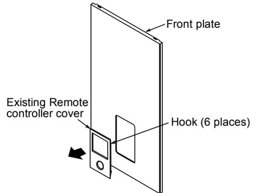
2. Press from front to fix the Remote controller cover on the front plate.
