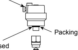
Apply some water based grease on packing surface before fix with shut off valve.
