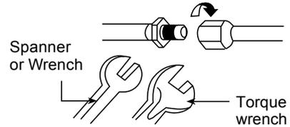
Be sure to use two spanners to tighten. (If the nuts are overtightened, it may cause the flares to break or leak.)
