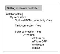
This is an application that connects the DHW tank to the indoor unit through 3-way valve before connect the solar water heater to heat up the tank. DHW tank's temperature is detected by tank thermistor (specified by Panasonic). Solar panel's temperature is detected by solar thermistor (specified by Panasonic).
