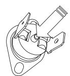
Use test pen to push this button for reset Overload protector (11).
