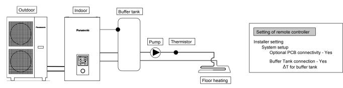
This is an application that connects the buffer tank to the indoor unit. Buffer tank's temperature is detected by buffer tank thermistor (specified by Panasonic). This system requires optional PCB (CZ-NS4P).
