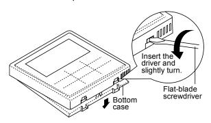
2. Remove the wiring between Remote controller and Indoor Unit terminal. Remove the bottom case from the Control board cover by loosening the screws. (3 pieces)
