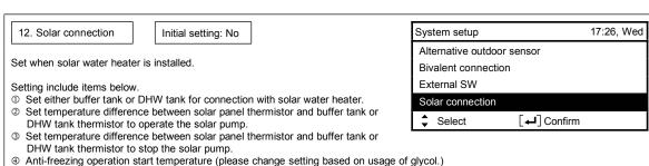
Solar pump stop operation when it exceeds high limit temperature (when tank temperature exceed designated temperature (70~90°C))
