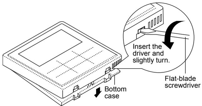
1. Remove the top case from the bottom case.
