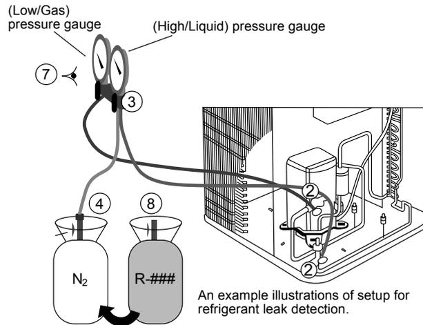
**Step 2: Refrigerant leak detection through Electronic halogen leak detector and/or ultrasonic leak detector:**
