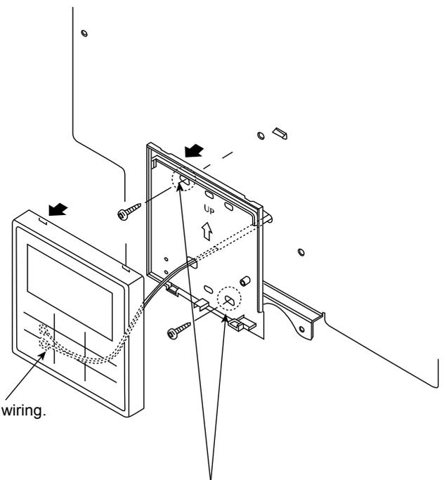
2. Disconnect the Remote Controller wiring.
