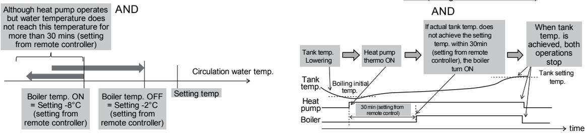
In Advanced Parallel mode, setting for both heating and tank can be made simultaneously. During operation of "Heating/Tank" mode, when each time the mode is switched, the boiler output will be reset to OFF. Please have good understanding on the boiler control characteristic in order to select the optimal setting for the system.
