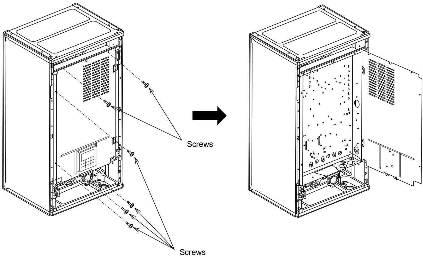
1. Remove 6 screws from the Control Board Cover.
