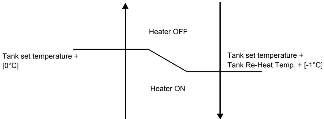
a) Tank heater Turn On condition:
