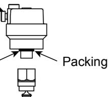
During reinstall Flow Sensor
