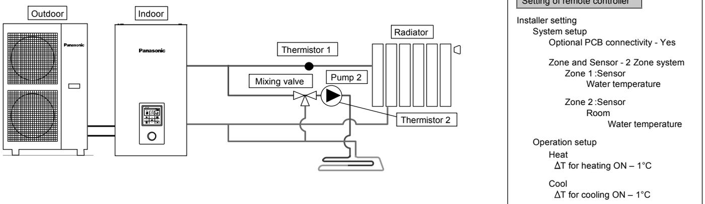
This is an example of simple 2 zone control without using buffer tank.
