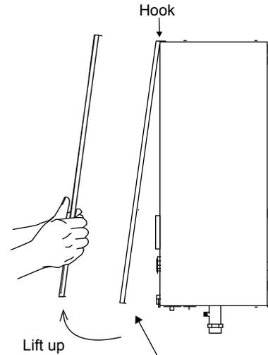
3. Hold the left edge and right edge of front plate to lift up front plate from hooks.
