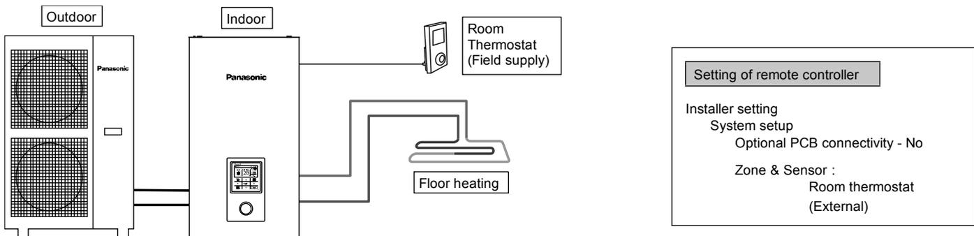
Connect floor heating or radiator directly to indoor unit.
