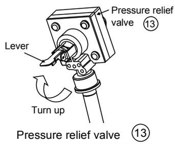
3. Start filling water (with pressure more than 0.1 MPa (1 bar)) to the Indoor Unit via water inlet. Stop filling water if the free water flow through Pressure Relief Valve drain hose.
