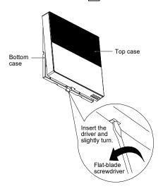
3. Reverse the steps 1 to 4 of section "Remove The Remote Controller From Tank Unit" to fix Remote Controller Case 4 on Tank Unit.
