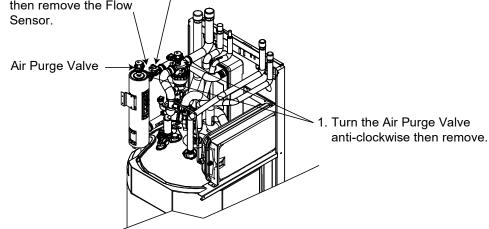
Mhen reinstall Flow Switch, ensure the arrow on the flow switch is parallel with the pipe shaft and is facing in the direction of flow.
