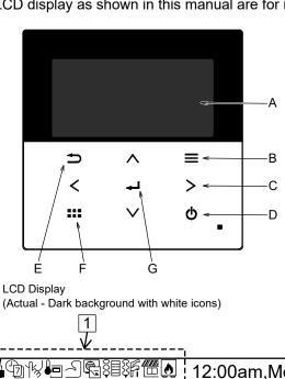
Name Function A: Main screen Display information Open/Close main menu B: Menu Select or change item C: Triangle (Move) D: Operate Start/Stop operation E: Back Back to previous item F: Quick Menu Open/Close Quick menu G: OK Confirm
