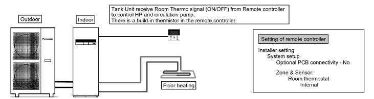
Connect floor heating or radiator directly to the Tank Unit.
