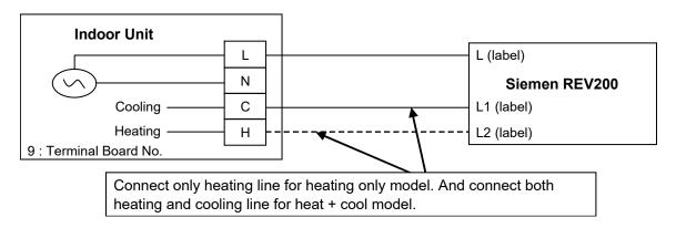
Wire Connection and thermo characteristic of Siemen RAA20:
