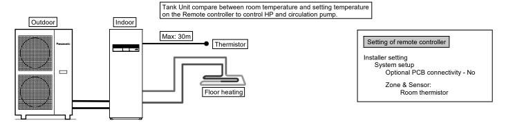
Connect floor heating or radiator directly to Tank Unit.
