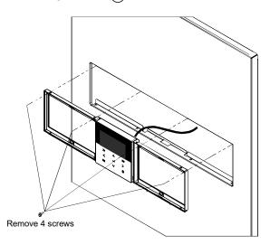
3. Remove the top case from the bottom case.
