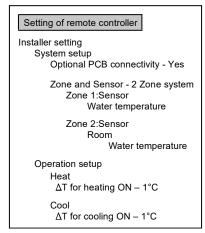
This is an example of simple 2 zone control without using buffer tank.
