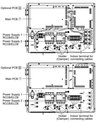
How to guide the optional cables and power supply cord (view without internal wiring)
