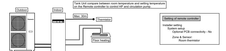
Connect floor heating or radiator directly to Tank Unit.
