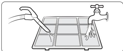
Clean the air filter with a vacuum cleaner or soft brush. If dust is too heavy, then rinse it with running water and dry it in a ventilated area.
