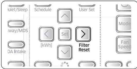
After cleaning and reassembling the air filter, be sure to reset the filter-cleaning reminder as follows:
