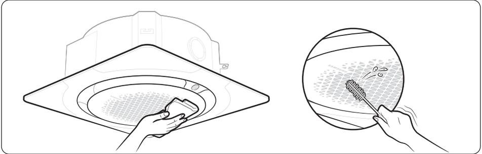
Wipe the surface of the unit with a slightly wet or dry cloth when needed. Wipe off dirt from odd-shaped areas by using a soft brush.
